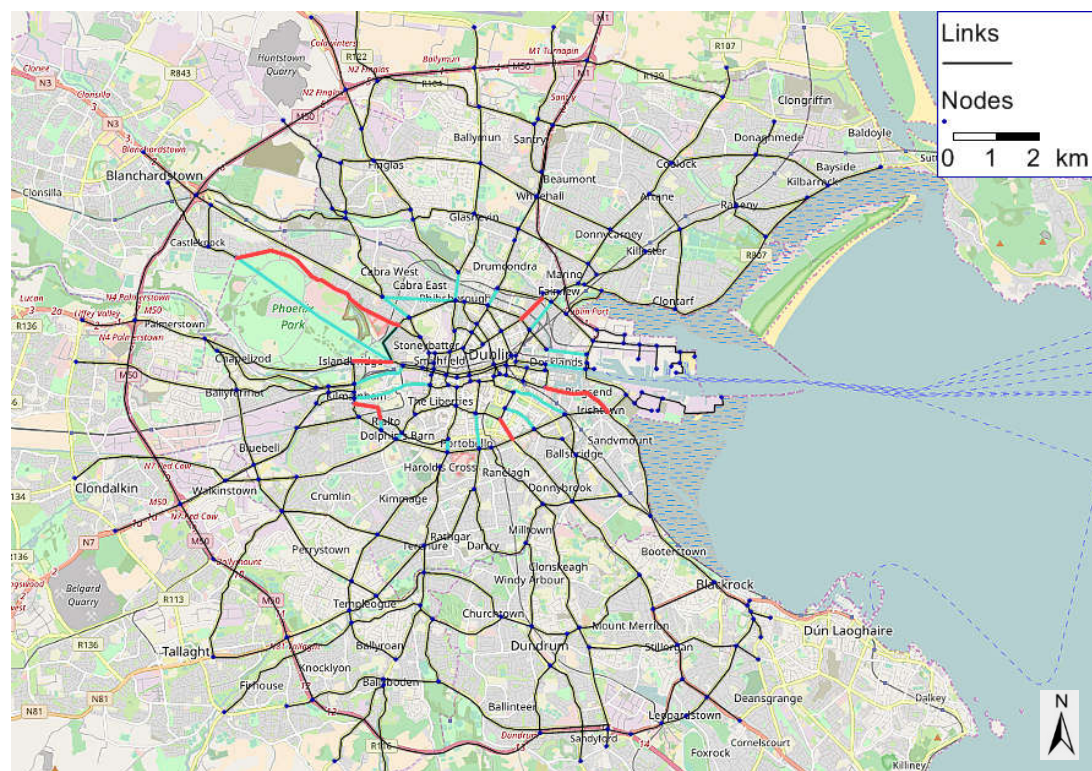
Figure 3-2: Links of calibration (blue line) and links that met the validation criteria (red line).
