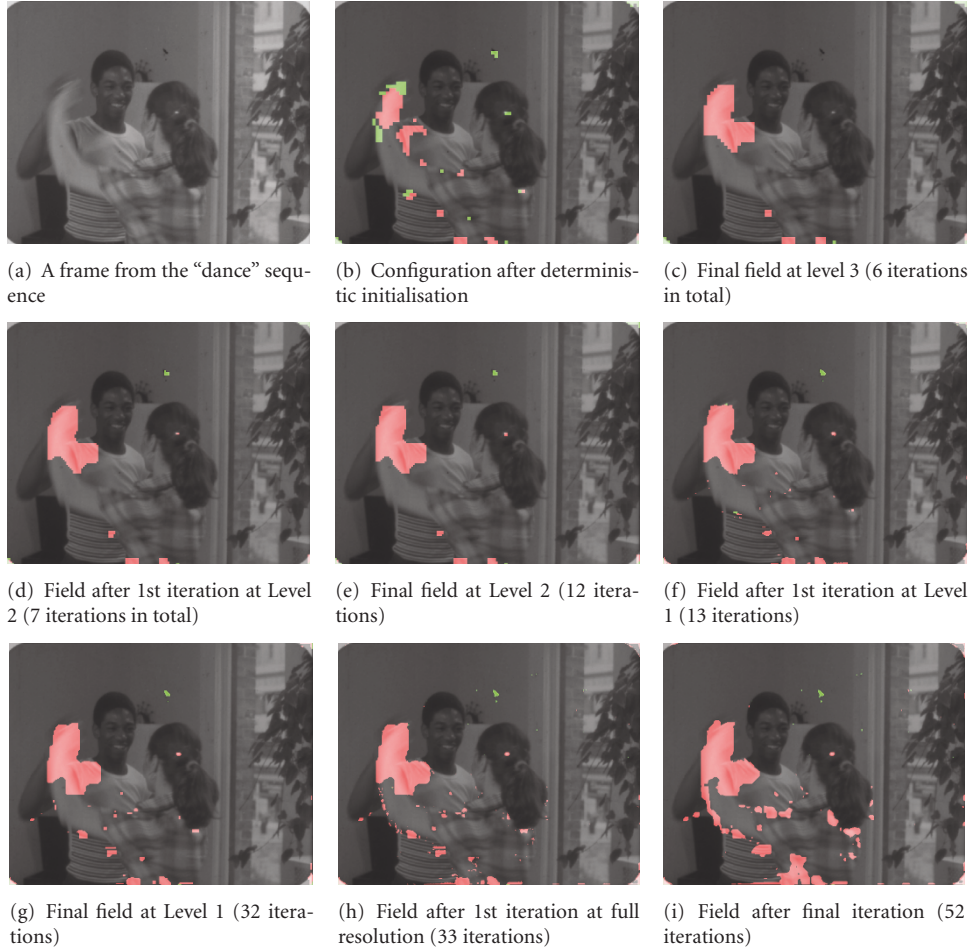
FIGURE 9: This figure shows intermediate values of the label field (PM—Red, Blotches—Green) at various iterations of the ICM optimisation process for a frame from the “dance” sequence. The standard parameter set is used (Section 5.2) and the value of \delta_t is 7. Level 0 corresponds to the full resolution; the resolution at level 1 is 360 \times 288 and so on. At the coarsest resolution (Level 3) the resolution is 90 \times 72 pixels.
