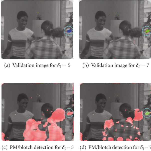
FIGURE 11: This figure illustrates how lowering the DFD threshold \delta_t results in a lower correct detection rate. The blue circle highlights a large blotch which is not detected at the lower threshold ((a) and (b))—correct detections in green, missed detections in blue). At the lower threshold this blotch is classified as PM ((c) and (d))—red for PM, green for blotches).
