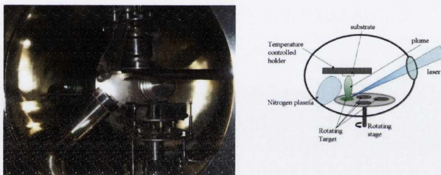
Figure 3.2 The PLD deposition chamber and a schematic view of the process.
