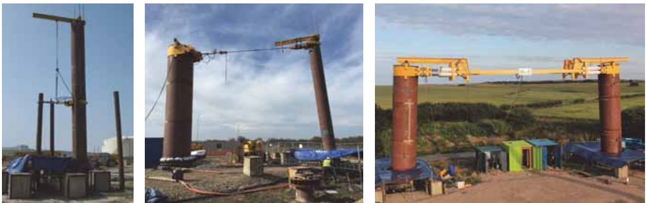
Figure 10: Images of the small ( D = 0.273 \text{ m} ), medium ( D = 0.762 \text{ m} ) and large ( D = 2.0 \text{ m} ) diameter test arrangements.
