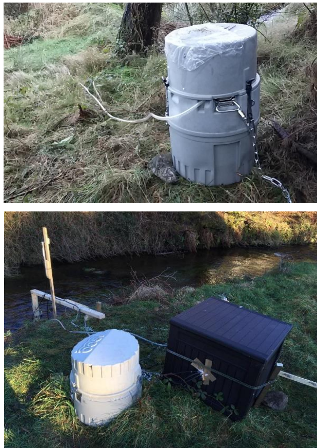
Figure 3.7 Automatic water samplers.
