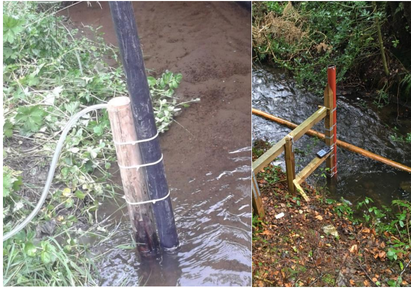
Figure 3.6 Water level sensors in the feeding rivers.
