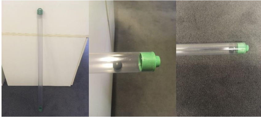
Figure 3.10 Water bailer used for sampling underground water.
