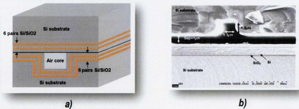
Figure 1-5: a) Schematic structure of hollow waveguide; b) SEM image of cross-section of hollow waveguide [19].
