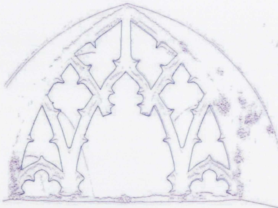
Figure 7.9 Athenry Dominican priory: nave west window from laser scan with overlaid vectors
