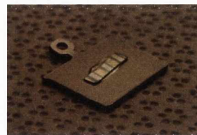
Figure 4.6 Si(100)/Au,Pt sample used for STM tip conditioning.
