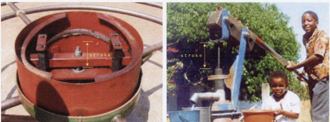
Fig 7.3: The interior of the PlayPump 's headgear, left (Obiols & Erpf 2008, p.21); and the Zimbabwe Bush Pump's headgear, showing the much longer travel of the pump mechanism, right (arrows and text added).
