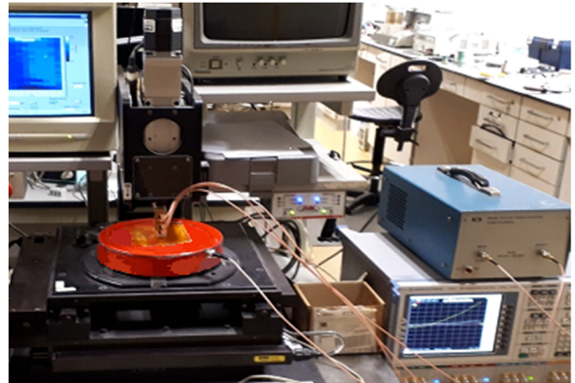
FIG. 2. Experimental setup for RF scanning using a micro-coil set as inductive sensors positioned within a 0.21 m diameter source coil. (not visible). The DUT is placed under the micro-coil and the z -height adjusted so as to scan as close as possible above the sample surface. Z -scanning or z -slicing can also be performed as an alternative data acquisition strategy.
