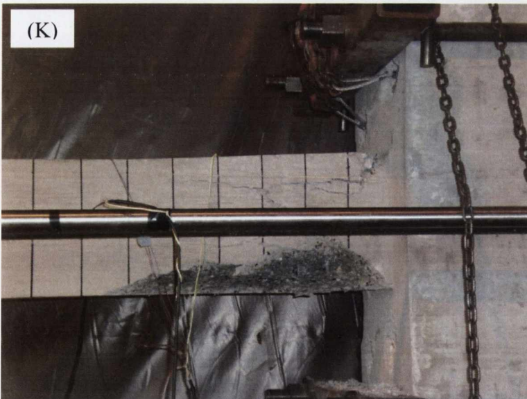
Figure 4.11: Photos: (I) & (J) Specimen JD5 & JD6 Post 1 st 60mm displacement, (K) Specimen JD5 Post 2 nd 60mm Displacement
