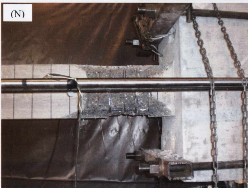
Figure 4.11: Photos: (L) Specimen JD5 Post 60mm Displacement Cycles, (M) Specimen JD1 Post 90mm Displacement Cycles, (N) Specimen JD5 Post 90mm Displacement Cycle
