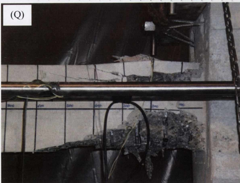
Figure 4.11: Photos: (O) Specimen JD6 Post 90mm Displacement Cycles, (P) & (Q) Specimen JD1 & JD6 Post 120mm Displacement Cycles
