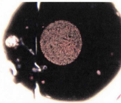
Figure 98. AgNW section on a PDMS tip. As can be seen in this dark field image the nanowire film appears quite opaque and relatively even.
