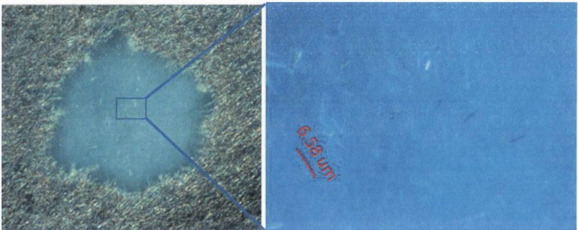
Figure 116. Images of the inked region after Test 2. The image on the left shows the AgNW network after inking. The image on the right is a higher magnification of the alumina after inking. As can be clearly seen there are still individual nanowires in this region and one is measured to be 6.6 \mu\text{m} long.
