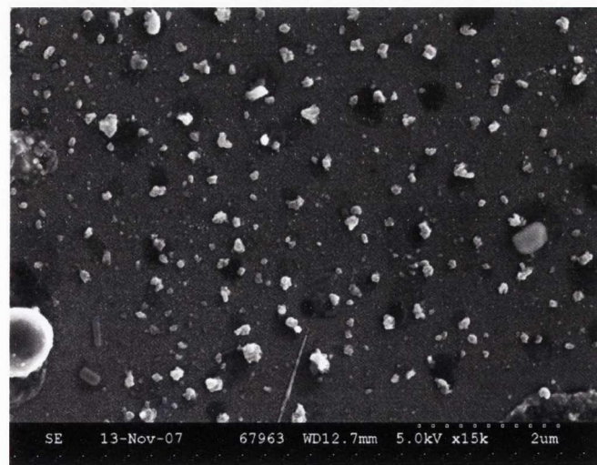
Figure 6.7 SEM images of silver deposited during confined laser ablation at 1.5 \text{ J cm}^{-2} at three different magnifications. The length scale is shown in the bottom right corner.
