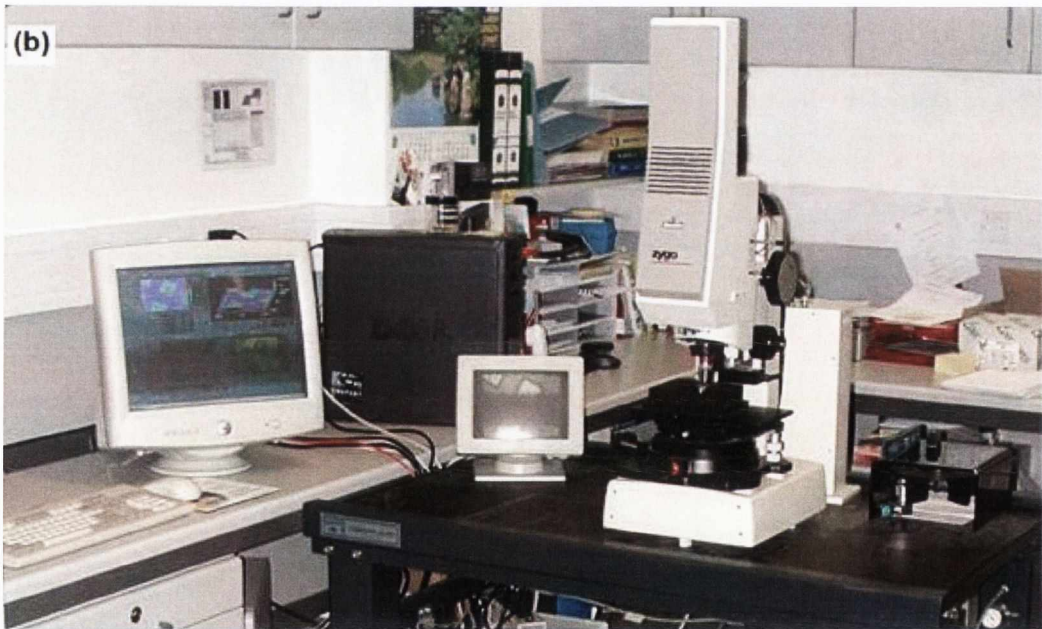
Figure 2.8: (a) Scheme of the functioning principle of a scanning white light interferometer. (b) Picture of the device used.
