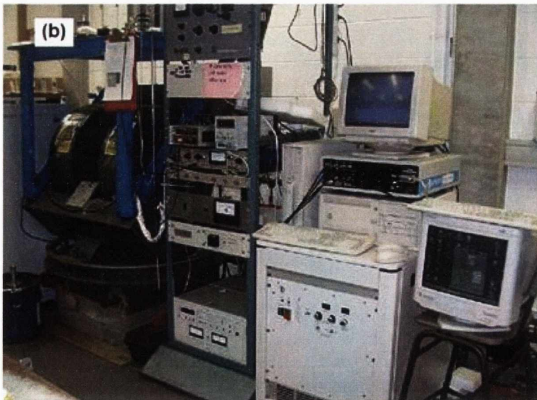
Figure 2.3: (a) Scheme of an electromagnet. (b) Picture showing the equipment setup used in most of the experiments with horizontal fields up to 1.5 Tesla.
