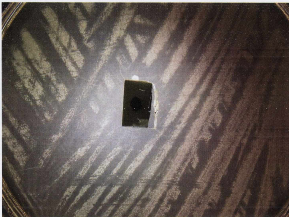
Figure 5.21: Ag / PANI thin film, which was prepared by electrodeposition onto ITO at 1 V for 2000 s, after exposure to pseudomonas aeruginosa bacteria for 11 days
