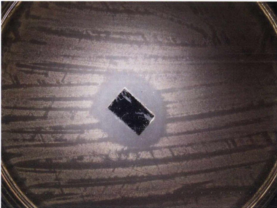
Figure 5.20: Ag / PANI thin film, which was prepared by electrodeposition onto ITO at 1 V for 1000 s, after exposure to pseudomonas aeruginosa bacteria for 11 days
