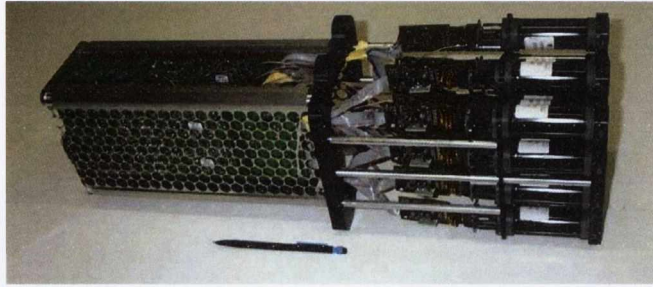
Figure 2.7: A single drawer contains 16 PMTs and the associated electronics.
