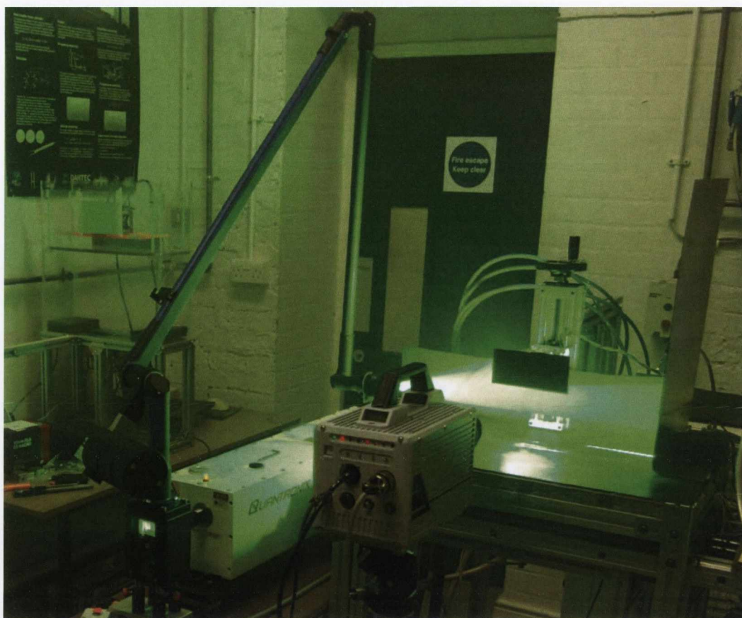
Figure 4.6 – Experimental setup for 2D-2C PIV testing, preliminary setup to configure beam stops to prevent reflections
