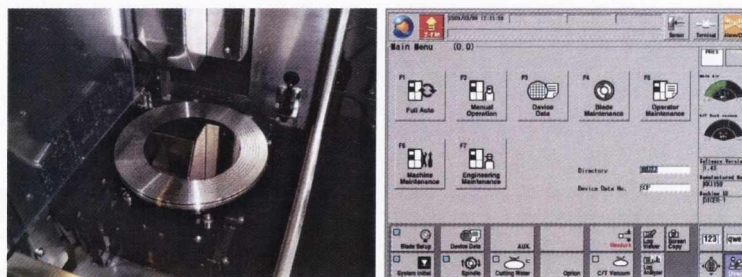
Figure C.7: Wafer loaded onto chuck table; C/T Vacuum button on lower right side
