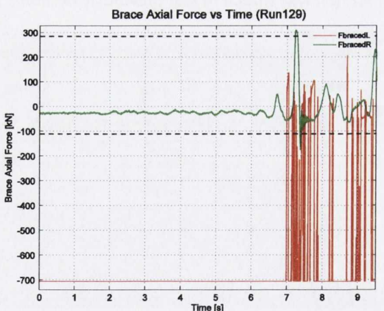
(c) Brace axial load time history for left (FbracedL) and right (FbracedR) braces. Dashed lines indicate yield and buckling capacities (based on characteristic strengths and measured brace section area).
