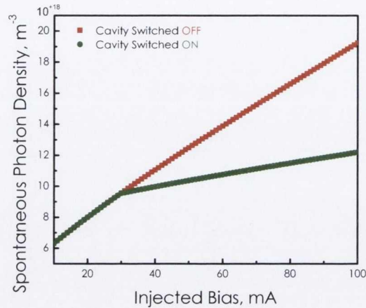
Figure 4.5: Simulated spontaneous photon density as a function of total injected bias, when the lateral cavity is switched on (green) and when it is off (red). A deviation in output power is seen at the output due to the clamping of carriers in this region.
