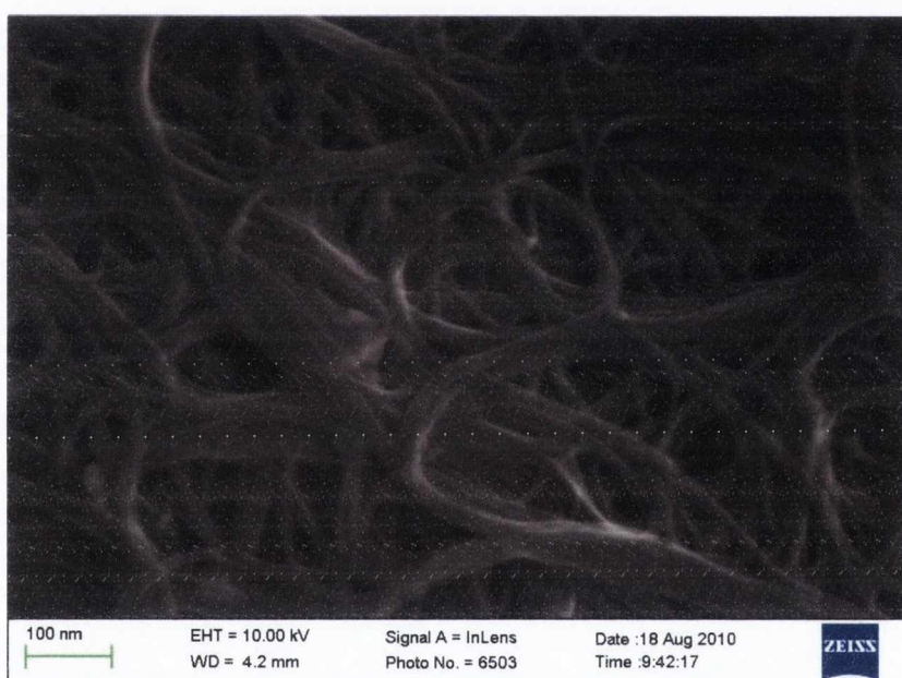
Figure 4.1 SEM image of the surface of a film prepared from Ijlin SWNTs in SDS/H 2 O. This image is representative of all the carbon nanotube films made in this study.
