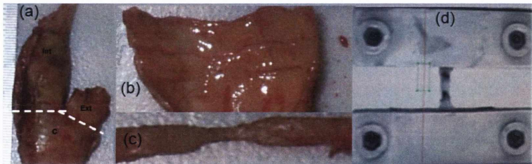
Figure 3.1: (a) Intact carotid plaque specimen. Dotted white lines show where specimen was separated into common (C), internal (Int) and External (Ext) carotid segments. Dog-bone shaped tensile specimen (b) before and (c) after sample is fully excised from common carotid segment. (d) Image from video-extensometer of tensile specimen clamped in tensile grips.
