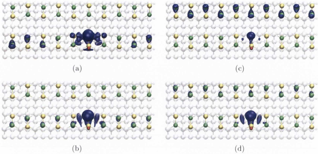
Figure 5.8: HOMO and LUMO states around the Fermi energy for the n -doped H_T configuration, calculated with periodic boundary conditions. A pattern modulation, corresponding to the first quantum well state, can be seen in the first row LUMO state (a). The magnitude of the pattern modulation is quite reduced in the HOMO (d) and LUMO (c) states on the second row and no standing wave pattern can be identified.
