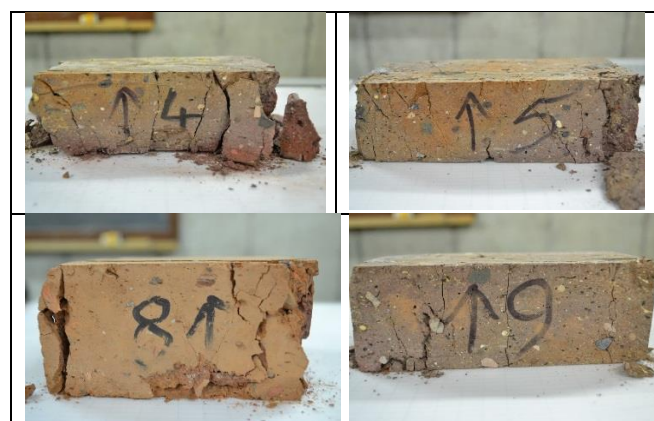
Figure 4. Failure modes of the bricks in the dome.
