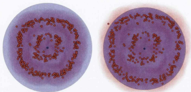
Figure 6.23: Comparison between the fitted (left) and original (right) tube diameter. The center of each bubble is marked using a red point, while the extent of each bubble is shown by a light red disc. The center of the tube is marked in blue while the extent of the tube is shown in light blue. The fitted tube radius covers the extent of each bubble, while the original tube diameter suggests the extrusion of bubbles out of the cylindrical container.
