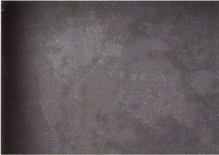
Figure 1.7: Photograph of the top layer of a 3D monodisperse aqueous foam of average bubble diameter 400 \mu\text{m} . The bubbles are seen to spontaneously form distinct crystal domains which are separated by disordered grain boundaries.
