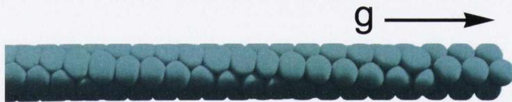
Figure 6.1: Graphic showing the ordering of monodisperse microbubbles within a cylindrical tube. The bubbles are seen to order in a regular, repeating structure. The nature of these ordered cylindrical packings will be examined in this proceeding chapter.
