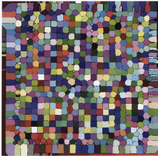
Figure 2.14: Application of the watershed transformation. Each connected domain is given a unique numeric identifier, corresponding to a unique colour.
