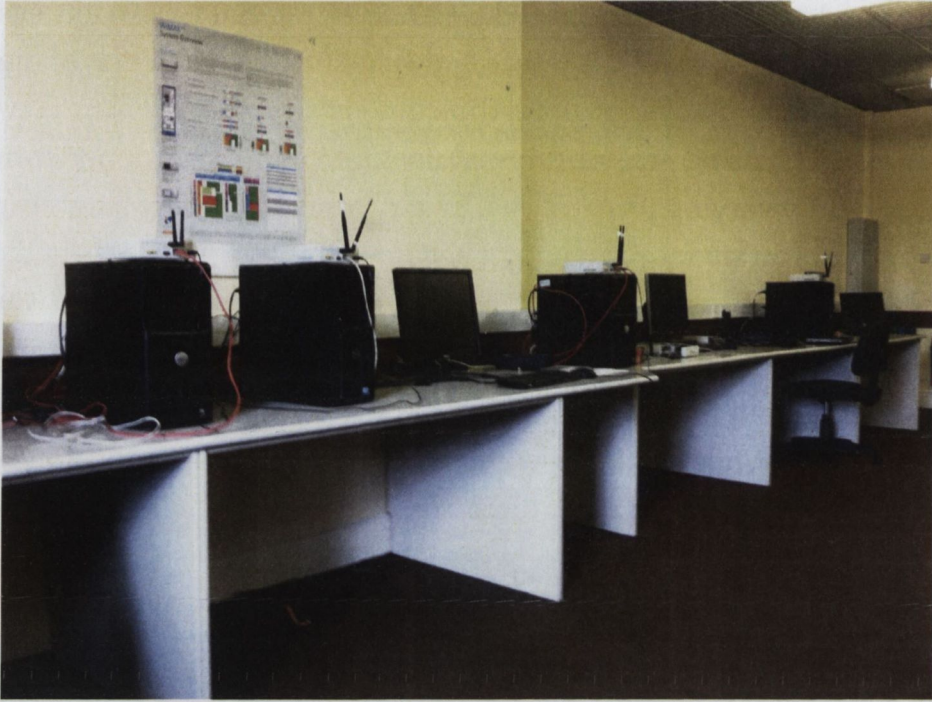
(a) Photo of CTVR testbed, featuring 4 Iris-GPP-USRP nodes.
