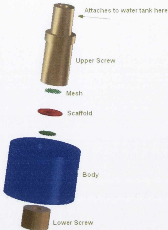
Figure 4.3 Exploded view of permeability rig (with thanks to Nicole Fisher for diagram)
