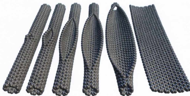
Figure 1.3: “Unzipping” a carbon nanotube to form a graphene nanoribbon. This figure is adapted from Ref. [49].
