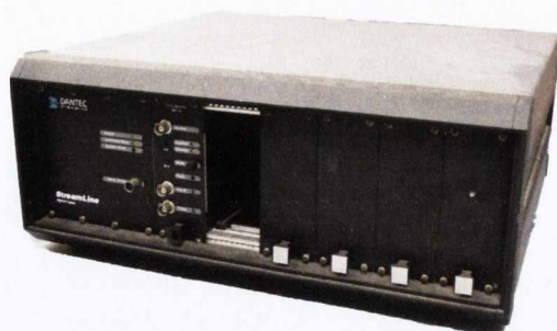
Figure 4.14: Dantec Dynamics 90C10 CTA Module housed in a Streamline 90N10Frame
