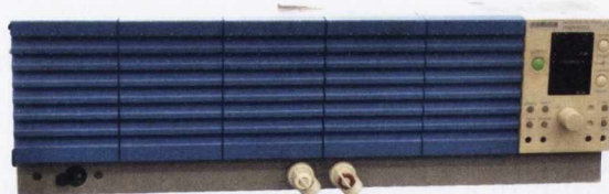
Figure 4.8: Kikusui PWR1600L 1600 W DC power supply used to heat impingement surface
