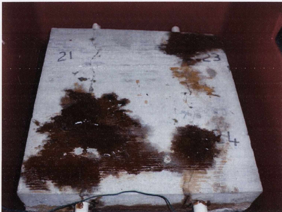
Figure 5.19. Staining of OPC+PFA slabs from pore fluid
