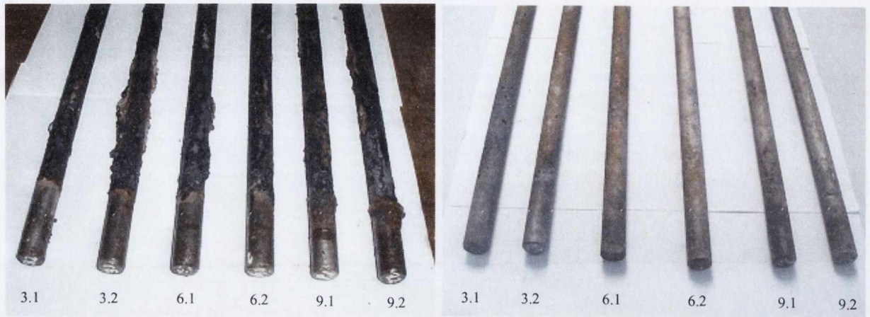
Figure 5.22. Steel reinforcing bars before and after cleaning according to ASTM G1-90
