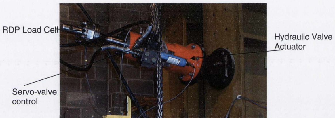
Figure 5.7(c) Load cell and RDP actuator mounted horizontally to the frame.
