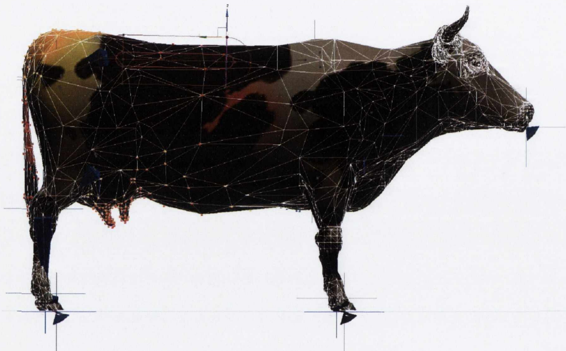
Figure 4.6: The red and yellow colours indicate which part of the mesh is influenced by the spine bone. A red colour indicates that the spine has the most influence on the movement of those particular vertices of the mesh. As the colour changes towards blue, the spine bone has less and less influence over the particular vertices.
