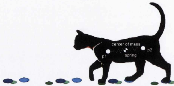
Figure 2.13: Two point masses are used in the simplified physics model to make the overall body movement look realistic. The footprints guide the position of the feet, the small circles represent the front legs, and the big circles represent the back legs (after [TvdP98]).
