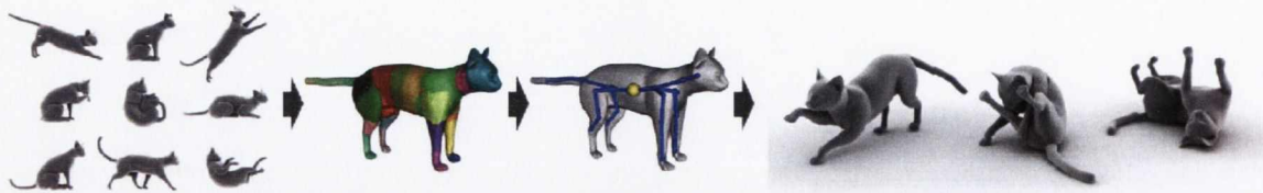
Figure 2.10: A set of input poses, mesh clusters representing rigid bones, computed skeleton (the yellow dot corresponds to the root of the hierarchy), and new poses created with this skeleton (Schaefer and Yuksel [SY07]).
