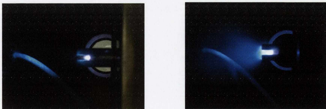
Figure 3.1: Digital camera photos of open-ended collar showing initial ablation plume (left) and -800 V discharge (right).
