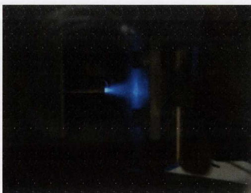
Figure 4.1: Plasma jet from conical nozzle discharge
