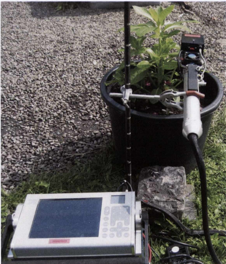
Plate 3.1 Measurement of photosynthesis using an infrared gas analyzer (Ciras 2, PP System).
