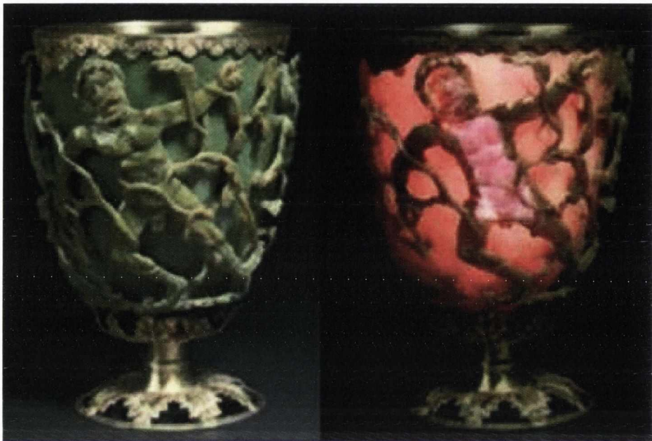
Figure 4.8: The Lycurgus glass cup appears green in reflected light and red in transmitted light due to dispersed gold nanocrystals.
