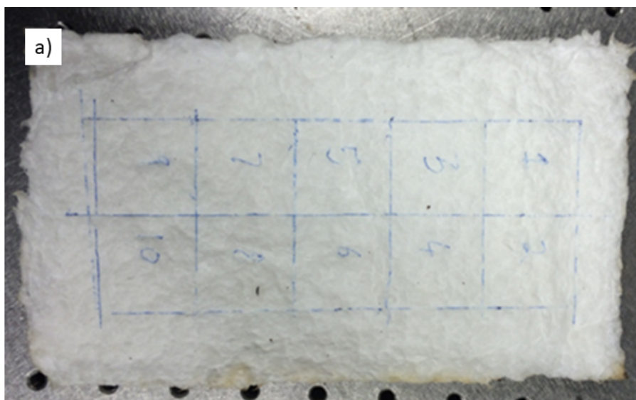
Fig. 3: Top view of a foam-formed fibrous structure that has dried but has not yet been cut into samples for further testing. The average height of the structure shown is 25mm.
