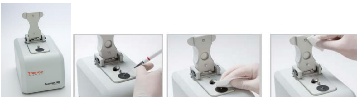
Figure 2.9: NanoDrop 2000c Clean down procedure post DNA measurement (Thermo Fisher Scientific, 2009)
