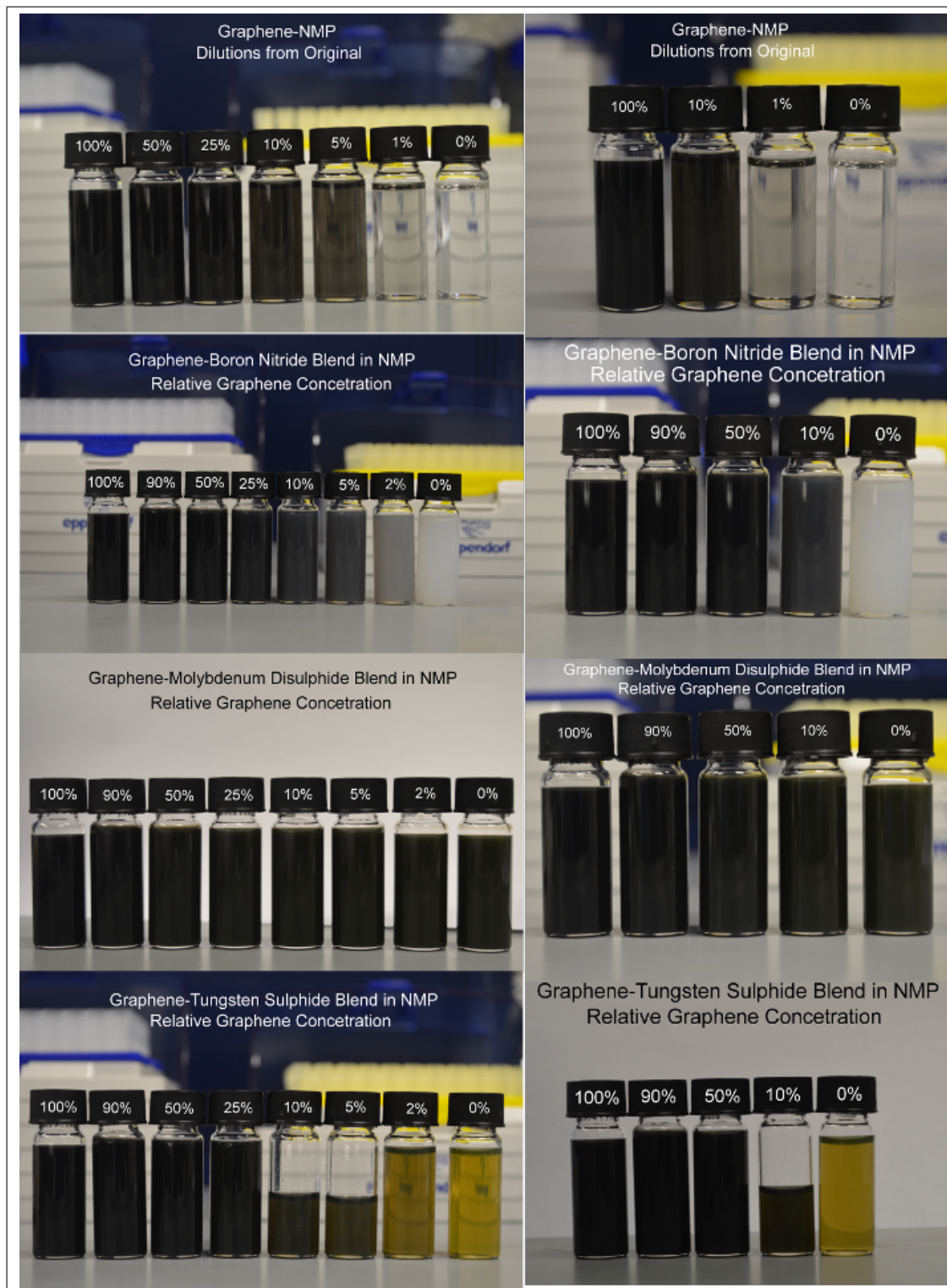
Figure 4.5: Blends of Graphene and Other 2D Materials in NMP
