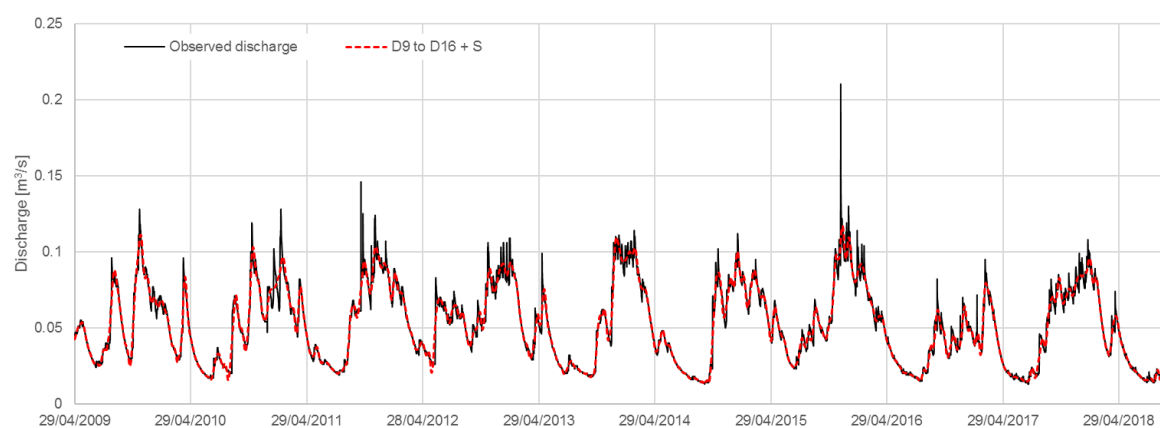
Figure 6.25: Low frequency signal (detail 9 to 16 + S) of db10 for discharge of Ballindine spring between 2009 and 2018.
