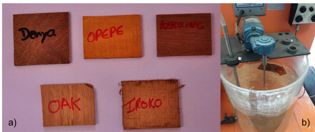
Figure 4.8: Wood chips (a) tested in a stirring tank (b).
