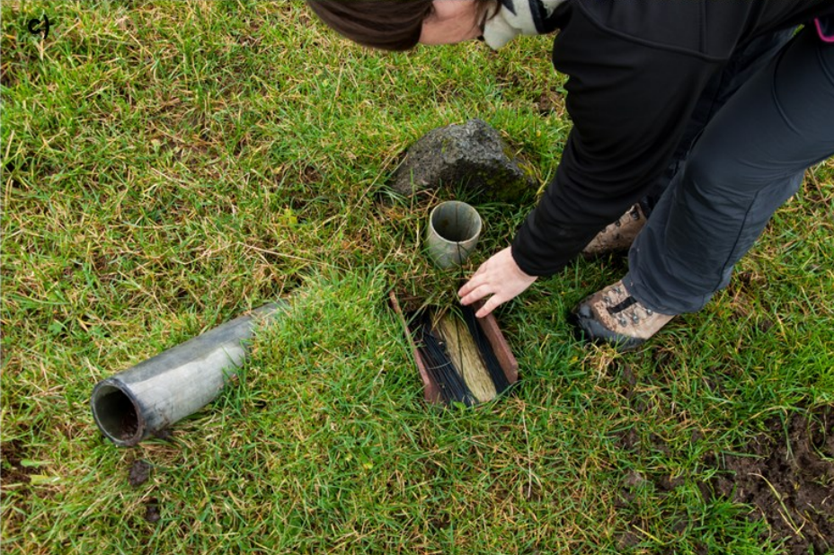
Figure A.8: Borehole BH1 during a single borehole dilution test (SBDT, a) and during automated sampling using an ISCO auto sampler (b) and borehole BH2 (c).
