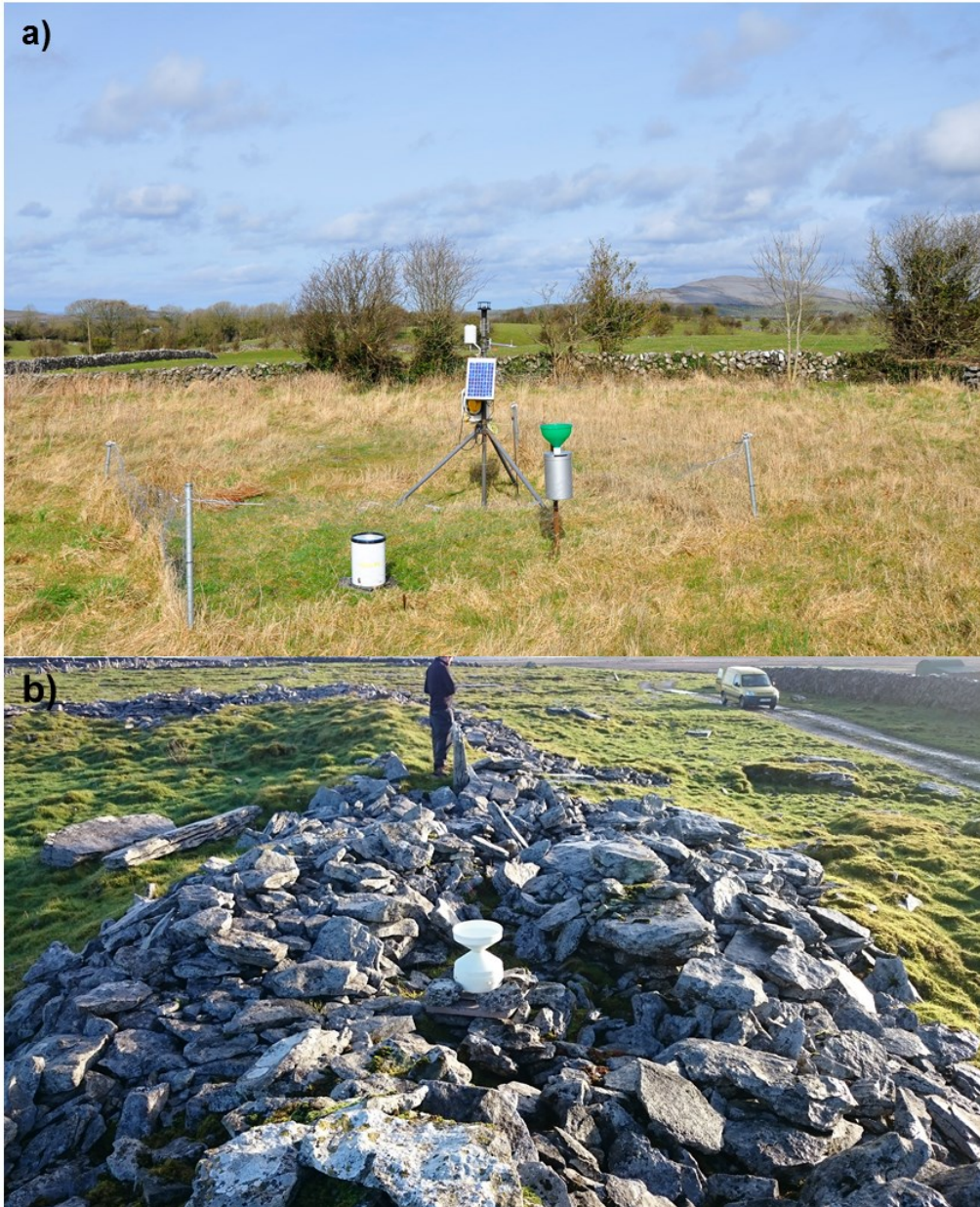
Figure A.7: Weather station (C1) at the BOEC including rainfall sampler and rainfall collector (a) and rainfall collector at FN (b).
