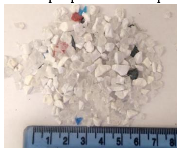
(b) PC: Varying morphology, similar to ABS with more sub-rounded particles and less fines.
