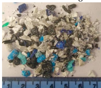
(a) ABS: Erratic morphology: flat, angular to cylindrical-smooth and rounded, rough-surfaced.
