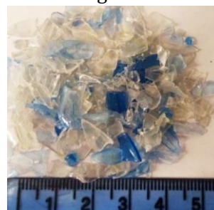
(c) PET: Flat, angular particles with smooth surfaces.
