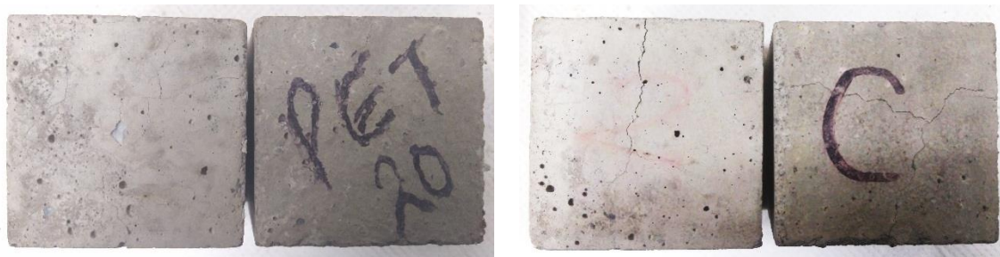
Figure 6. A representative sample of specimens after salt-crystallization cycling showing superficial hair cracks. Left-20% PET. Right-control mortar.
