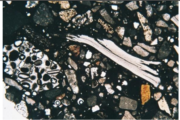
Figure 3. Coarse PET (jagged) and limestone aggregate (left) showing a good bond with the hydrated matrix (opaque). 2X natural light.
