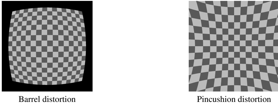
Figure 1: Two types of common lens distortion types. To the left: Barrel distortion. This type folds the image inwards and introduces black regions on the outside where image information is missing. To the right: Pincushion distortion. This type expands the image outwards and the outer edges of the image disappear.
