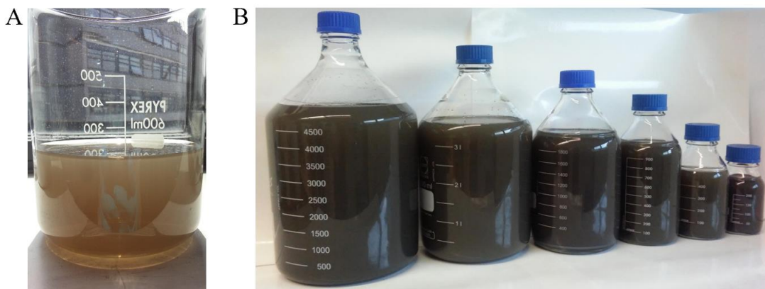
Fig.4.2. Images of impurities collected after pretreatment (a) and exfoliated WS_2 after the shearing stage (b). 30
