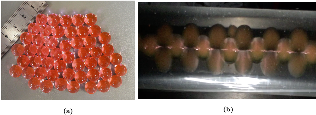
Fig 6.1: Possible future experiments about rotational columnar structures of soft sphere may be performed with hydrogel spheres. (a) shows an image of such hydrogel spheres. (b) is an image of a (4, 2, 2) structures assembled of hydrogel spheres involving rapid rotations with a lathe.
