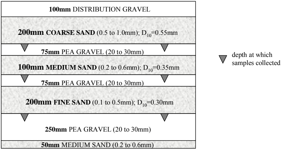
Fig. 2. Schematic cross-section through stratified sand filter.
