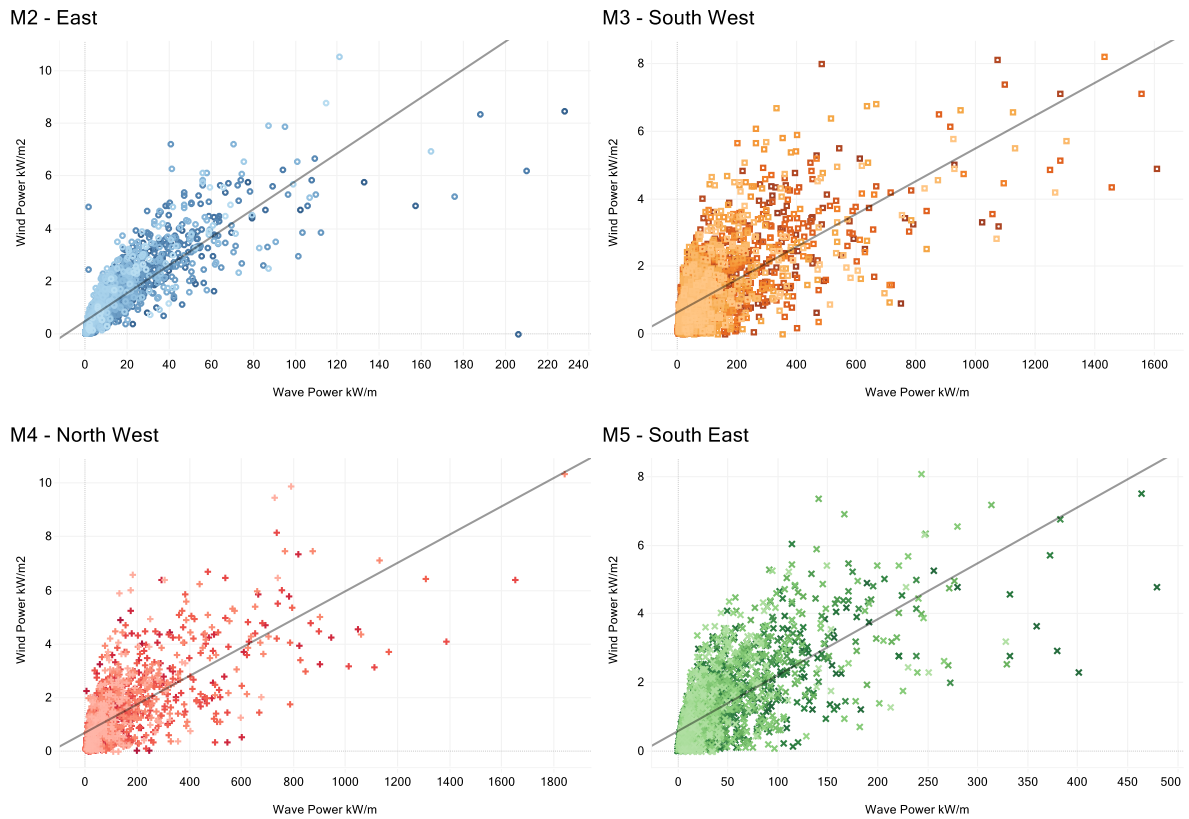
Figure 8: Scatter plots at zero time lag for potential wind and wave resource during the study period
