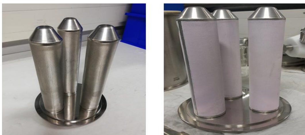
Figure 5. 10: Filters of the Mini-Glatt fluidized bed dryer before (left) and after (right) spray coating, highlighting material lost to the filters during the process due to small batch sizes.
