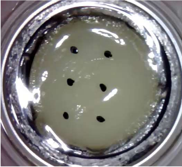
Figure A2.1 Flexcell plate well showing 6 dot pattern for strain testing
