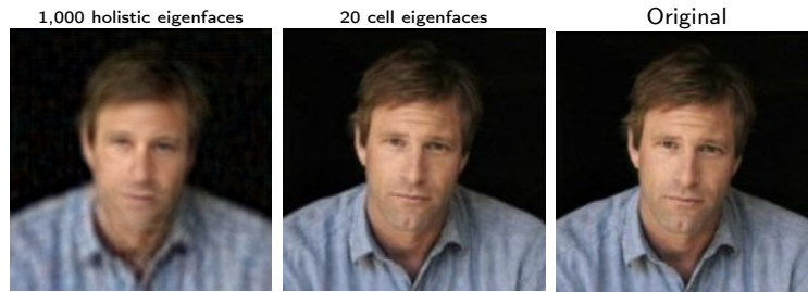
Figure 4.3: Reconstructed sample from LFW dataset using 1,000 holistic eigenfaces (with 13.2:1 compression ratio) compared to 20 cell eigenfaces (with 15:1 compression ratio). One can note the better reconstruction quality obtained when using CPCA despite the higher compression ratio.
