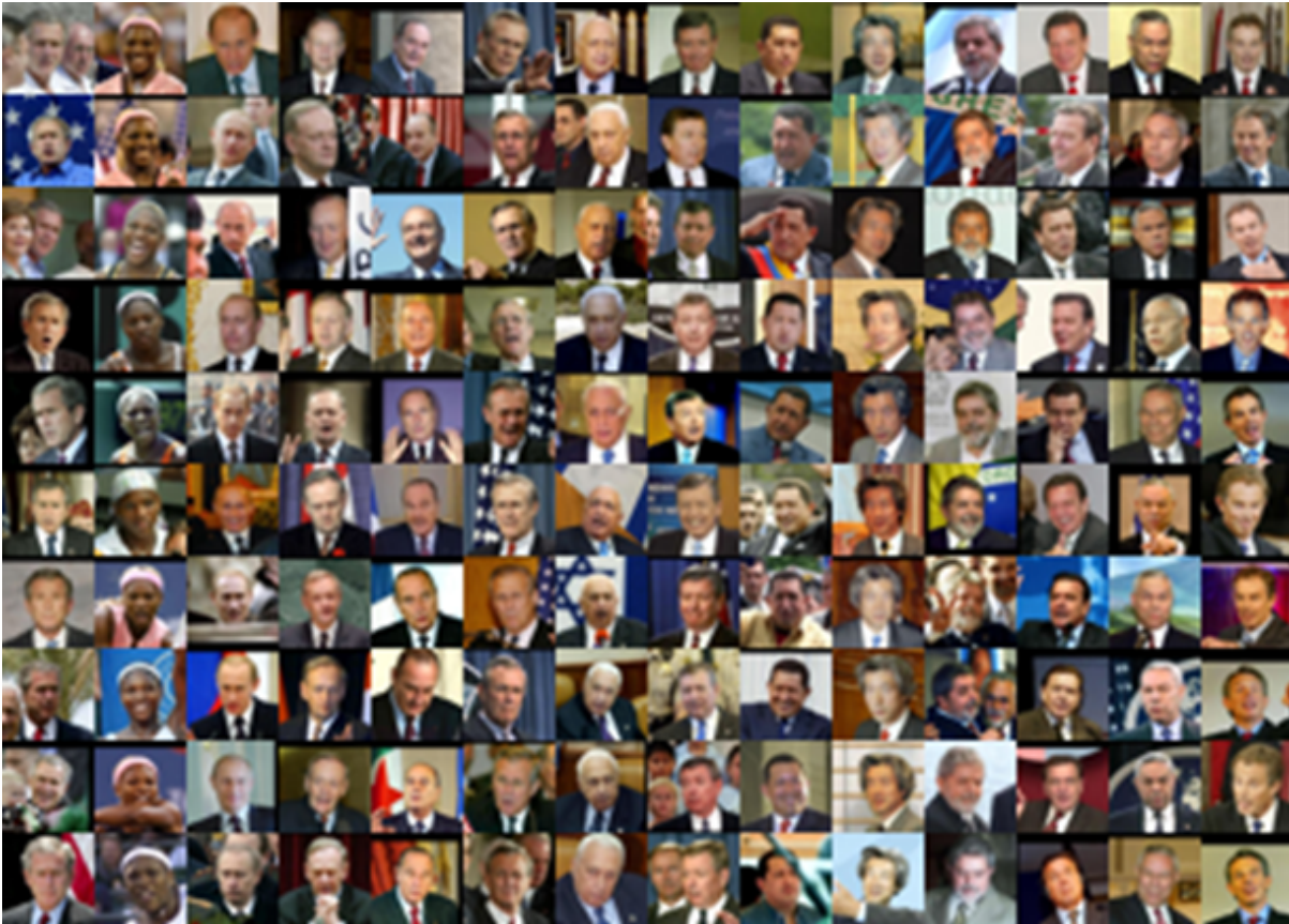
Figure 5.3: Downsampled face images using bicubic interpolation from 250 \times 250 pixels down to 25 \times 25 pixels. This depicts the main challenges that can occur in an image including scale, rotation, expression, illumination and background variations.
