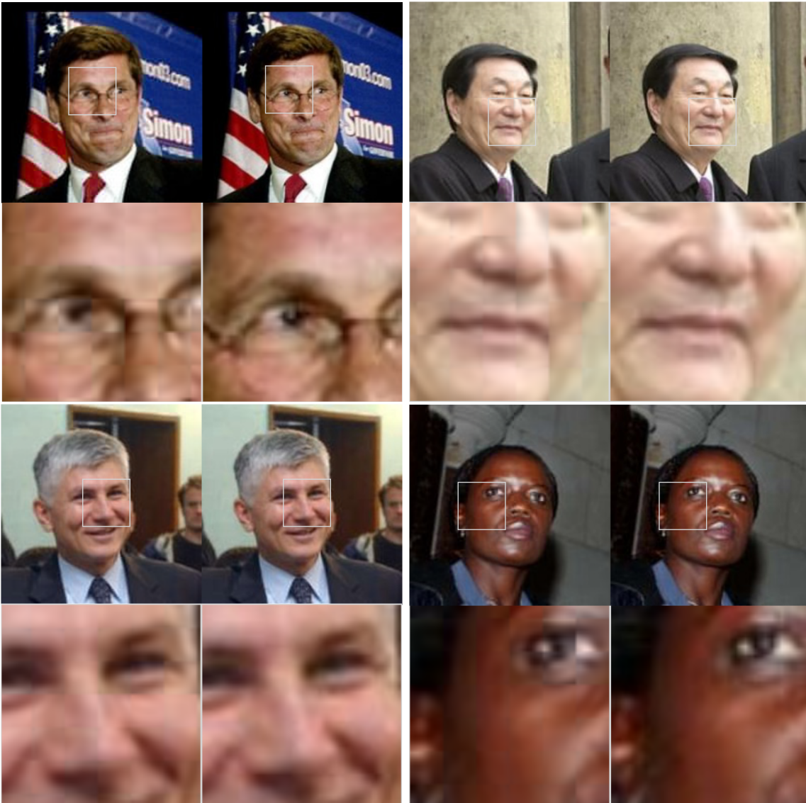
Figure 4.2: Comparing original samples from LFW dataset (right counterparts) with their reconstructions (left counterparts) when using 20 eigencells. Note the block artefacts in the zoomed areas.
