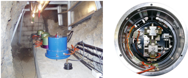
Fig 4: The sensor vault at MACI station, Morro de la Arena, Canary Islands ( Photo courtesy of Neil Ziegelman, Albuquerque Seismological Laboratory). (right) – Interior of a seismometer showing E/W and N/S sensors.
