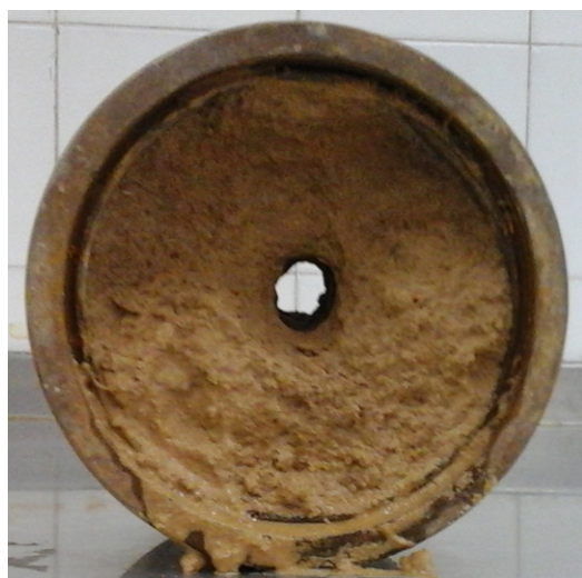
Figure 5. Uniformity of the eroded hole observed for SP-compacted 1% MK10–soil specimen after test completion
